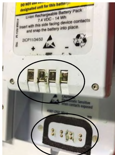
Unacceptable residue and corrosion build up
